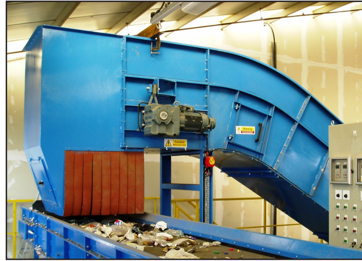
Infeed Conveyor onto Picking Belt.
