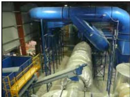
The equipment and plant installed gives the flexibility to the customer to handle logs and produce virgin wood chip, and accept woodchip or sawdust from other suppliers depending on market conditions and raw material supplies. Any of these raw materials can then be taken and fed by bucket loader into the plant in-feed system.
